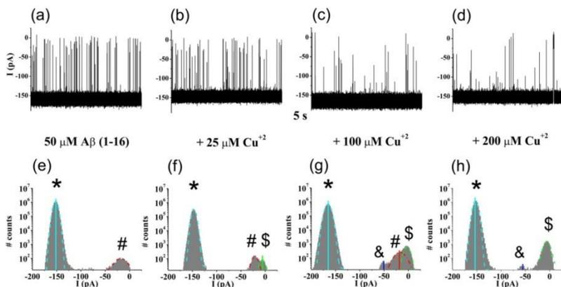
**Figure VI.2.2.1.** Typical single-channel current traces reflecting the uni-molecular interaction between the human Aβ<sub>1-16</sub> peptide with a α-HL pore, in the absence (panel a) and presence of *trans*-added Cu<sup>2+</sup> at various concentrations (panels b, c and d) [13].
