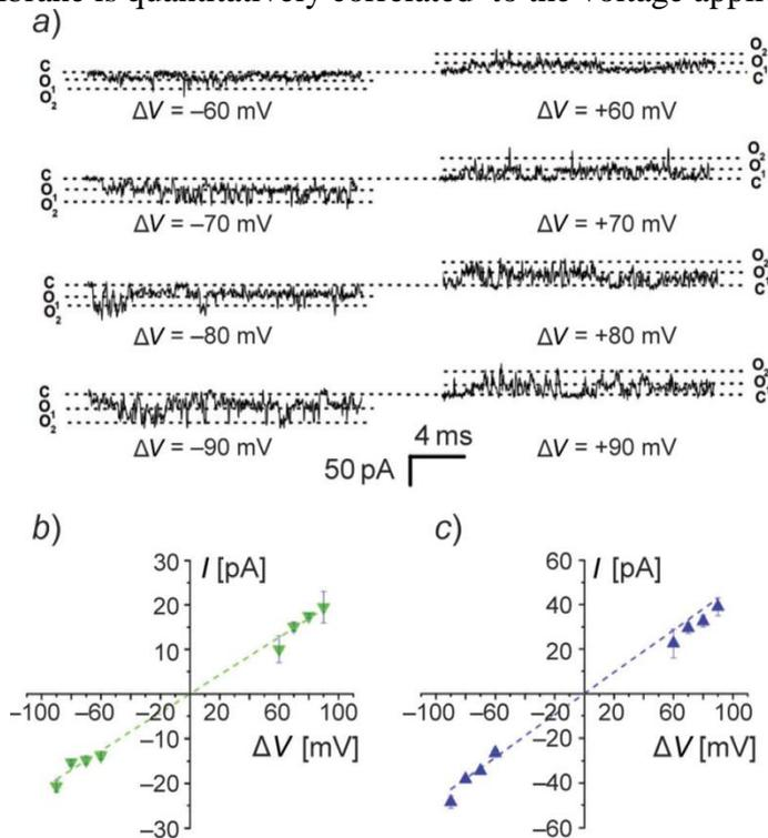
**Figure VI.1.1.1.** (a) Fluctuations of the ionic current recorded after added a 5  $\mu$ M of trichogin GAIV peptide in *cis* side of the lipidic membrane. Diagrams of the ionic current corresponding to the first conductive state  $O_1$  (b) and the second conductive state  $O_2$  (c) showing the ohmic behaviour of such ionic channels [11].
