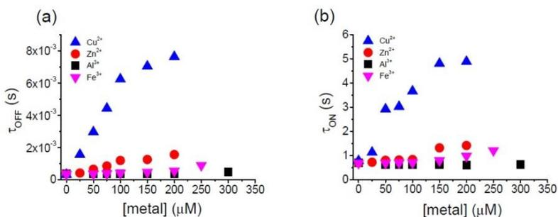
**Figure VI.2.1.4.** Dwell times  $\tau_{\text{off}}$  and  $\tau_{\text{on}}$  dependence of the metal ions concentration added in the system [13].
