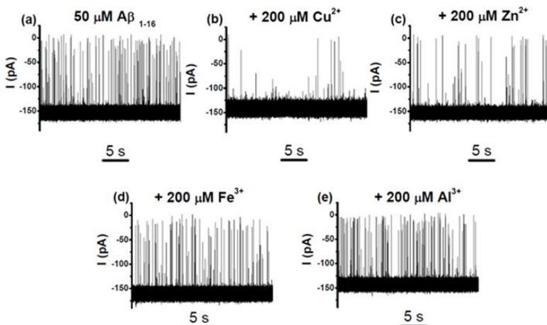
**Figure VI.2.1.2.** Fluctuations of the ionic current induced by the reversible interactions between the human peptide  $\text{A}\beta_{(1-16)}$  and the  $\alpha\text{-HL}$  pore in the absence of the metallic ions (a) and the presence of  $\text{Cu}^{2+}$  (b),  $\text{Zn}^{2+}$  (c),  $\text{Fe}^{3+}$  (d)  $\text{Al}^{3+}$  (e) ions [12].
